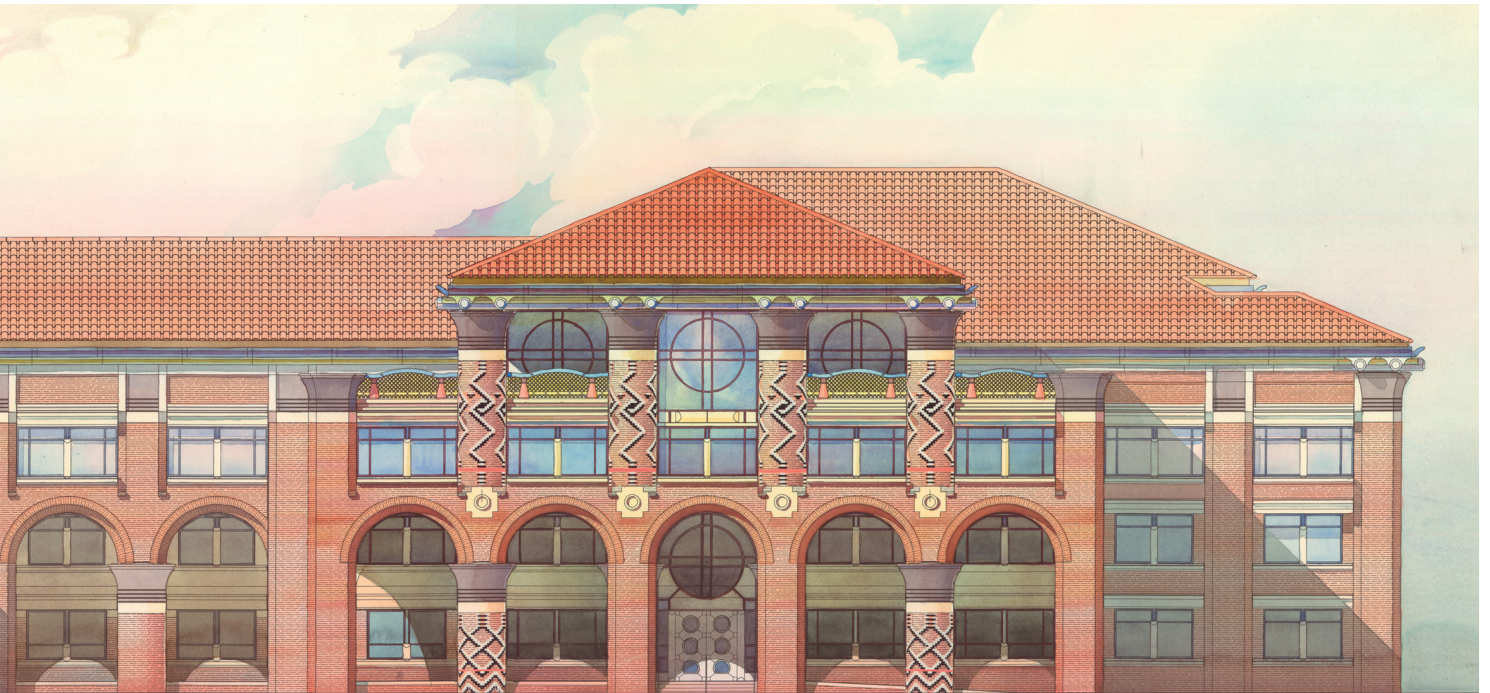
The southern portico to Duncan Hall that is illustrated above, presents a double-volume space, denoted the Meeting Room No. 1. It occupies the honorific position of a Balcony of Appearances located directly over the Main Door. This room is framed by the round columns on the Ground Floor. These columns also frame the three arches needed to signify the tridentine spatial flow that debouches from them through the Delta, into the Ocean of the Campus-City. The whole, honorific, composition is further reinforced by being inscribed with some of the Event Horizons of the Republic of the Valley, whose spatial narrative will be found inside the building.
