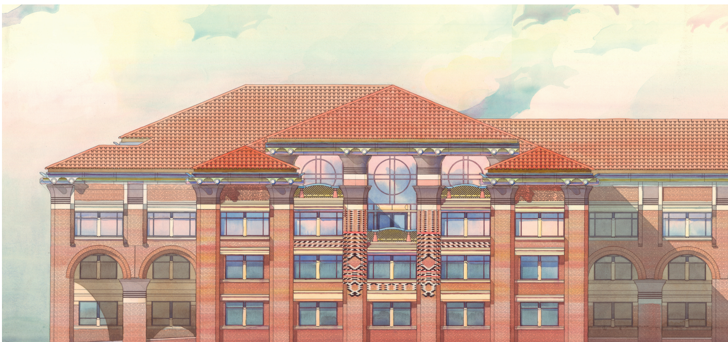
The plans of Duncan Hall shown on pages 27-14 to 27-15 describe how it is composed from two pavilions having bi-axial symmetry. Two of these 'wings', or arms, touch and make the nave-like internal street. The five remaining arms are divided at their ends into two pavilions framing three balconies to a main central pavilion. These fractured ends disguise the bulk of this new, air-conditioned deep-plan building-type and bring it into scale with the buildings erected in the first half of the 20C.
